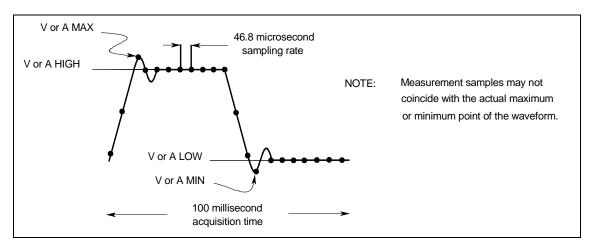
Figure 5-5. Default Front Panel Measurement Parameters
